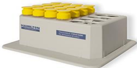
FIGURE 3: Exchangeable Hamilton thermoblock adapter for heating of the MAP-suspension in the Hamilton AutoLys M 1.0 tubes (the Hamilton heating block has to be mounted on an Eppendorf Thermomixer comfort or ThermoStat plus heater).
